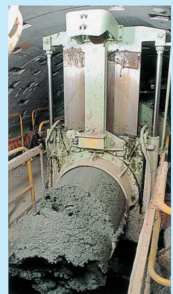
Excavated soil discharged from the screw conveyor
