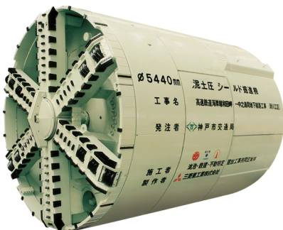
▲ Shield machine for the Kobe municipal subway
